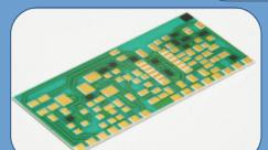
Substrate with AgENIG metallization, plated through-holes and printed resistors for a peak detector.
