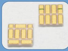
Substrate for a miniature TEC cooler. Use of AgENIG metallization with .0025" thick silver deposits and 0.35 m $\Omega$ /sq resistivity allowed current carrying capacity in excess of 10 AMP.
